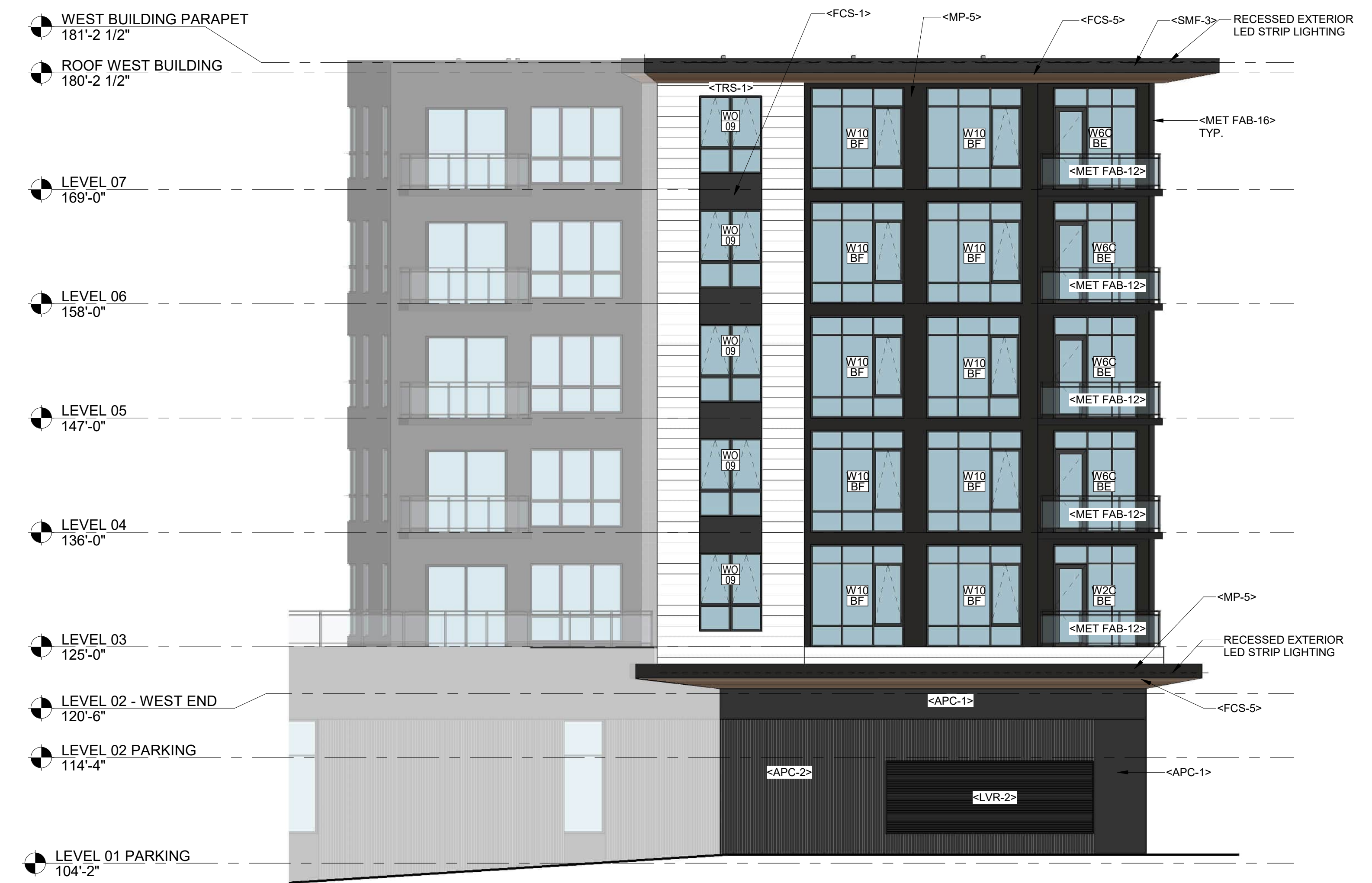
2 BUILDING B - NORTH ELEVATION 1/8" = 1'-0"
