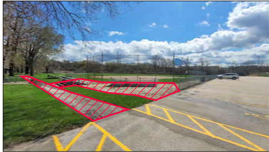
EXISTING PARKING AND ACCESS PATH. ELEVATE AND REPAVE. ADD CONCRETE PADS FOR DUGOUTS
